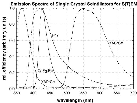
**Fig. 1** Normalized cathodoluminescent spectra of single crystal scintillators for S(T)EM.
