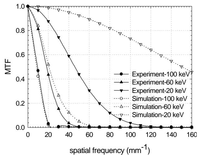
**Figure 2** Modulation transfer function of the YAG:Ce single crystal screen for different incident electron beam energies.
