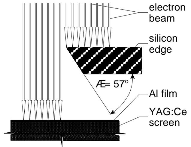
**Figure 1** Outline of an arrangement for unit step image creation by using the edge projection method.
