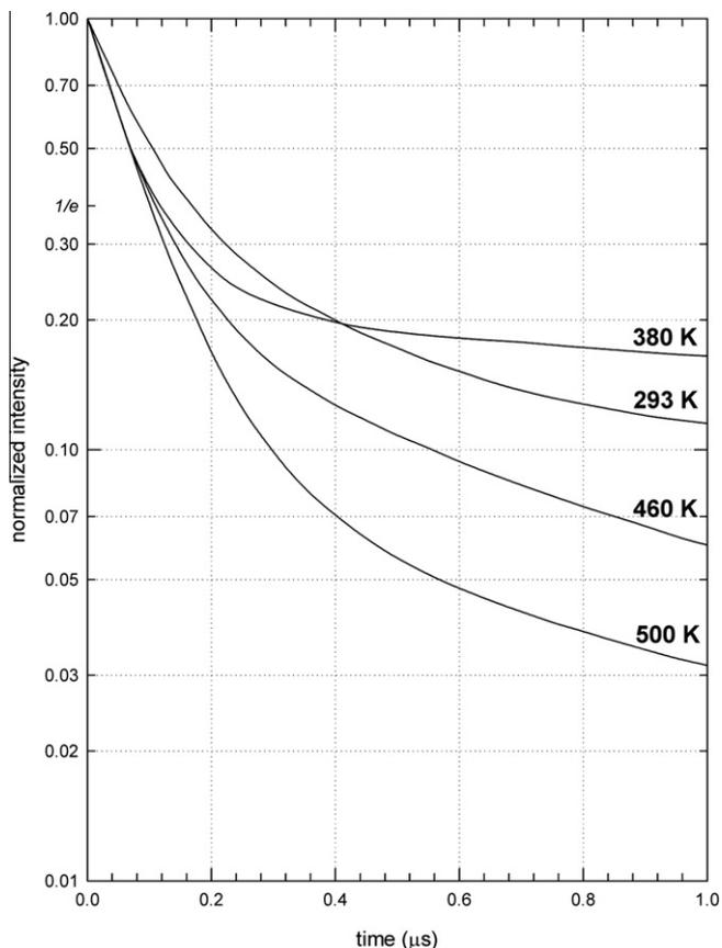
Fig. 5. Influence of the specimen temperature on the cathodoluminescence decay of YAG:Ce single crystal scintillators.
