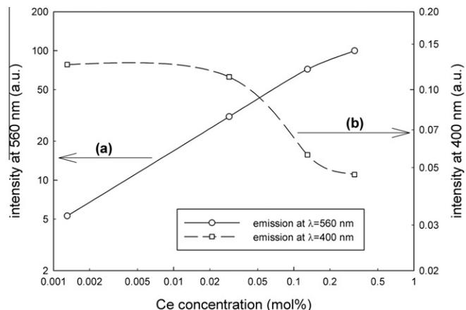
Fig. 7. Influence of Ce concentration in YAG:Ce single crystal on the (a) characteristic CL emission from the activator (560 nm), and (b) CL emission from the defects or the impurities at (360 nm) related to the maximum of the characteristic emission.
