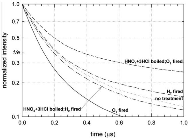
Fig. 8. Cathodoluminescence decay characteristics of YAG:Ce single crystals with different treatment conditions.
