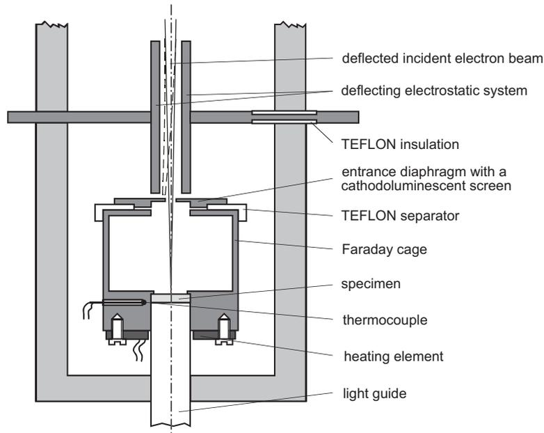
**Fig. 2.** Specimen chamber arrangement with the blanking system. The specimen was positioned at the face of the light guide and the signal was guided toward the detection unit.
