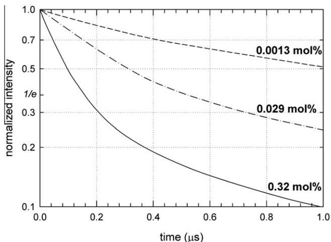
Fig. 6. Cathodoluminescence decay characteristics of YAG:Ce single crystals with different Ce concentrations.
