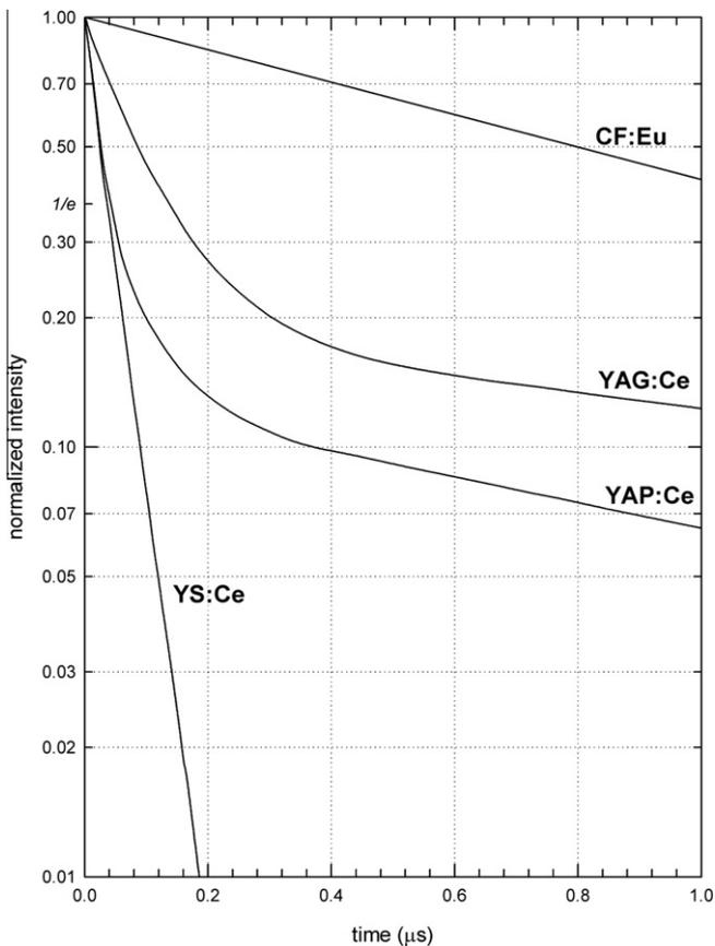
**Fig. 3.** Decay characteristics of single crystal scintillators for SEM. Excitation pulse duration 10  $\mu\text{s}$ .
