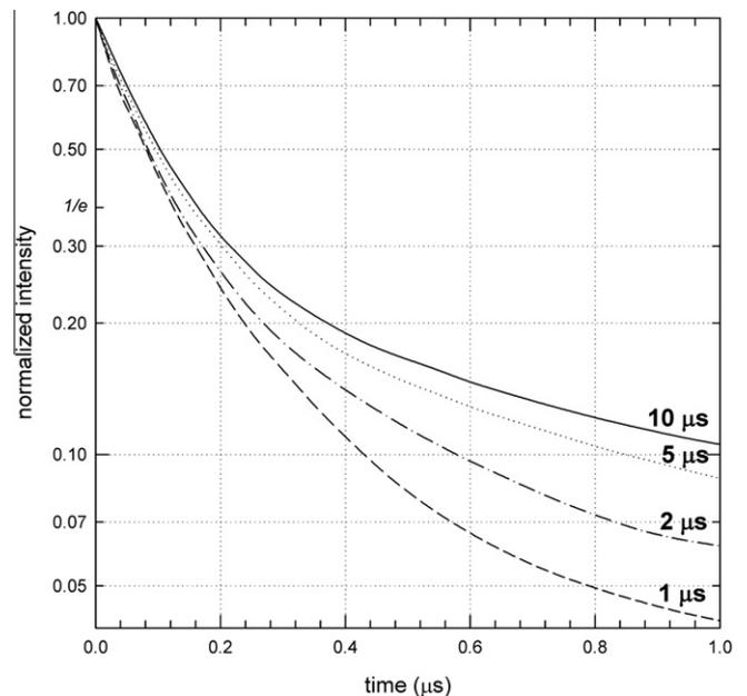
**Fig. 4.** Influence of the excitation pulse width on the cathodoluminescence decay of YAG:Ce single crystal scintillators.
