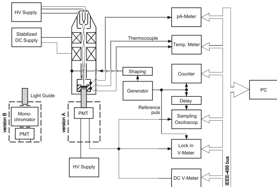
Fig. 1. Equipment used for CL property measurements.
