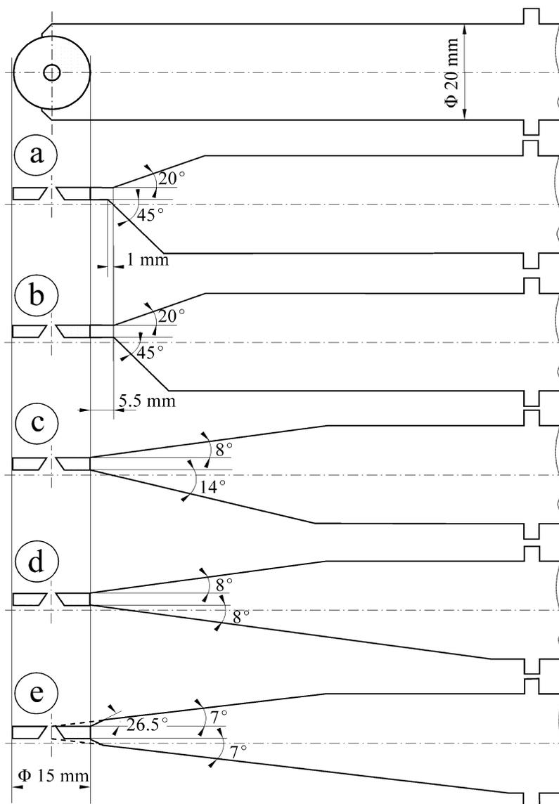
Fig 2. Schematic drawing of the geometry of key configurations during optimization of BSE scintillation detector S 4000 (Hitachi).
