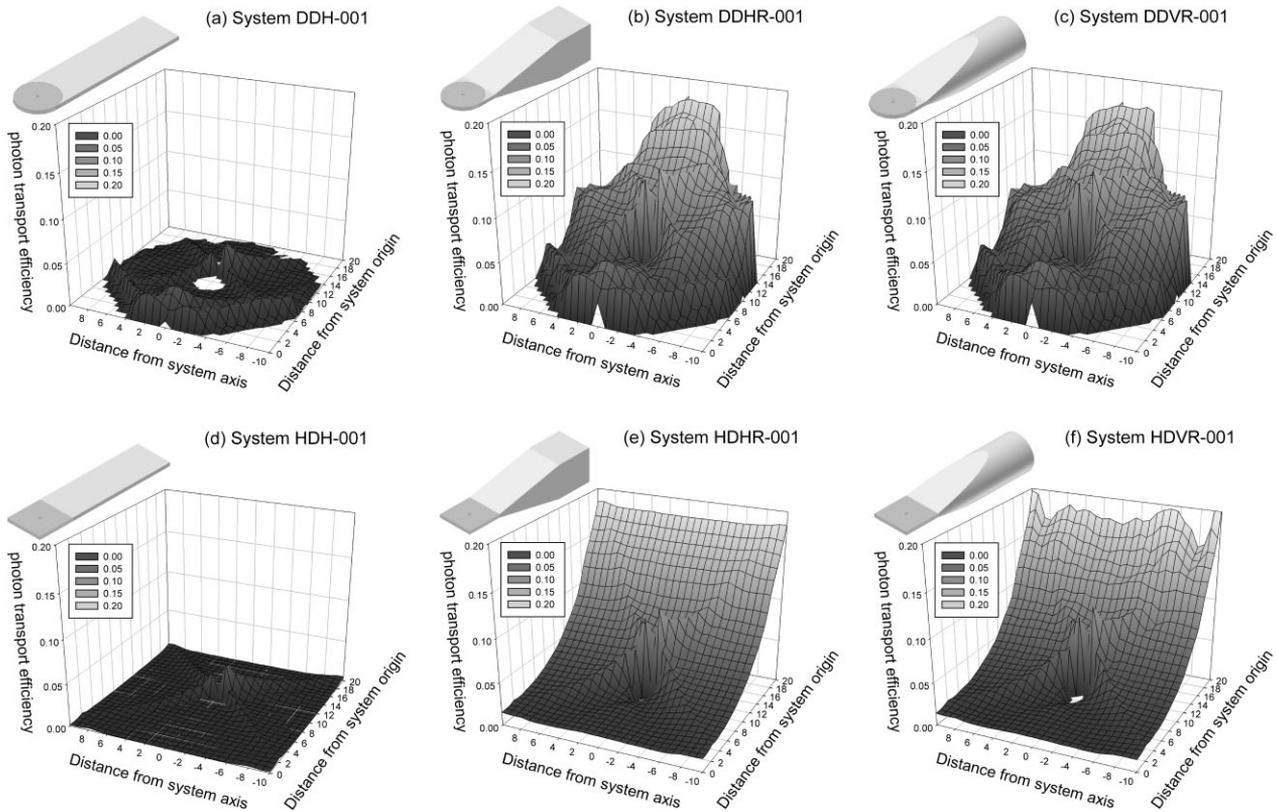
Fig 1. Photon transport efficiency in dependence on the point of excitation on the scintillator surface for different shapes of scintillators and light guides.
