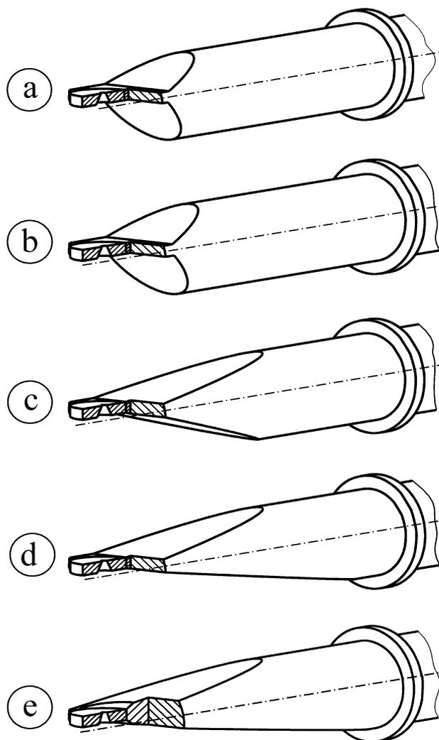
Fig 3. 3D images of the S 4000 BSE scintillation detection systems. Efficiency is improving from the basic (a) geometry to the final (e) geometry.
