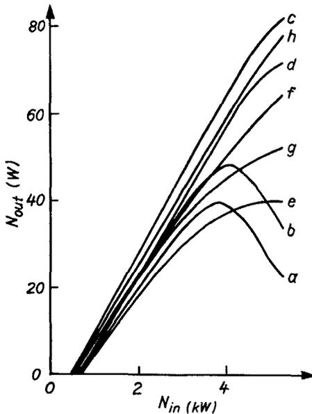
Fig. 3. CW output of the YAG rods  $\varnothing 6 \times 75$  mm. Absorption edge of the filter: a, b, c, d, e, f: 350 nm; g, h: 500 nm.  $R_{\text{out}} = 92\%$ , resonator length: 400 mm. Radius of the rear mirror: a, b, c, d, g, h: 5 m; e, f:  $\infty$ . Annealing: a, e, g: in  $\text{O}_2$ , followed by  $\text{H}_2$ ; c, f, h - in  $\text{H}_2$ ; d - in vacuum (crystal doped with  $3 \cdot 10^{-4}$  wt % Fe)
