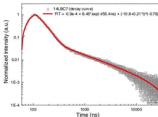
Fig. 1. Scintillation decay of GLGAG:Ce under 50 ns e-beam excitation. The solid line is convolution of instrumental response (not shown) to excitation pulse with the decay function consisting of one-exponential and a power-law terms,  $I = a + b.e^{-t/\tau} + (c+d.t)^{-p}$ .
