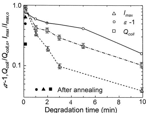
Fig. 5. The irradiation induced metastable states: time evolution of the total collected charge  $Q_{\text{coll}}$  (□), the dispersion coefficient  $\alpha$  (○) and the value of the photocurrent at the transit time  $I_{\text{max}}$  (Δ), also given are the values after anneal at 370 K for 10 min (●▲■). The lines are drawn as guides for the eye.
