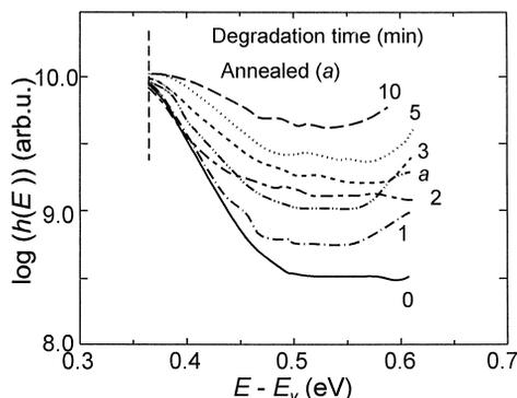
Fig. 6. The irradiation induced metastable states: time evolution of the metastable DOS function in the time interval  $t \in (0, 10)$  min, also given is the DOS after anneal at 370 K for 20 min (— · — · —).
