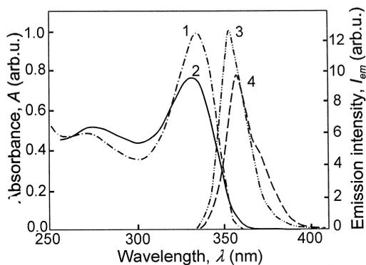
Fig. 2. Absorption spectra of PMPSi in tetrahydrofuran solution (curve 1: - · -) and in the solid state (curve 2: ———). Curves 3 (- · · -) and 4 (—) represent luminescence spectra in tetrahydrofuran solution and in the solid state, respectively.
