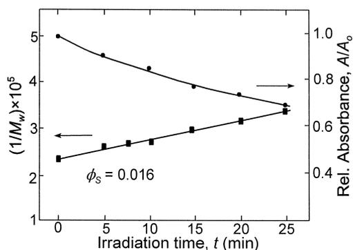
Fig. 3. Reciprocal value of the molecular weight of PMPSI vs. irradiation time ( $\lambda = 350$  nm)(■).  $\phi_s$  represents the quantum efficiency of polymer main chain scission. The lines are drawn as guides for the eyes.
