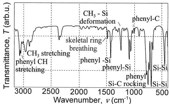
Fig. 1. Infrared spectra of PMPSi.
