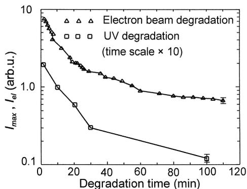
Fig. 4. The time evolution of the degradation both for the UV (Xe filtered, 75 W) radiation (□) and electron beam (10 kV, 1 nA) (Δ). The lines are drawn as guides for the eyes.
