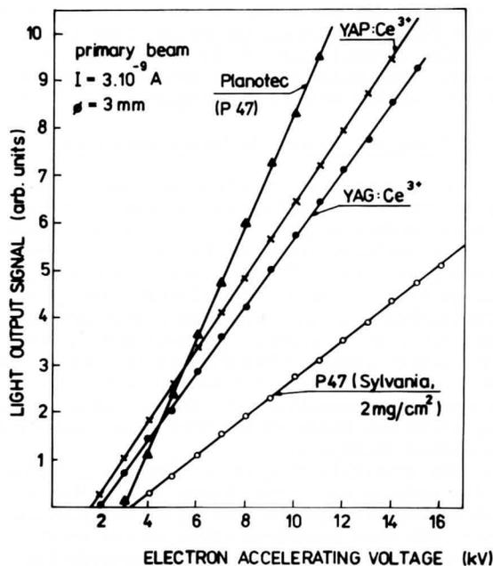
Fig. 2. Light output signal of single-crystal and P 47 powder scintillators plotted as a function of accelerating voltage.  $I$  - electron beam current,  $\phi$  - diameter of primary electron beam.
