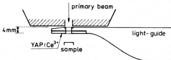
Fig.11. BSE detector with YAP:Ce<sup>3+</sup> single crystal.
