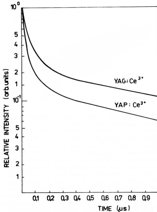
Fig. 4. Luminescent decay characteristics of single-crystal scintillators. Excitation pulse duration 10  $\mu$ s, concentration of  $\text{Ce}^{3+}$  ions  $1 \times 10^{-2}$  at %. Treated in oxygen and hydrogen atmosphere at 1500  $^{\circ}\text{C}$ , 3 h.
