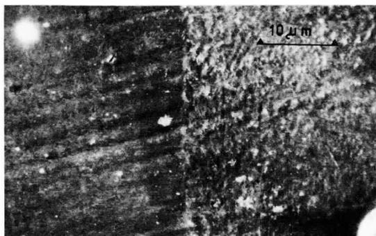
Fig.9. Secondary electron image. Left-hand side - copper, right-hand side - Cu-Zn alloy, specimen current  $1 \times 10^{-10}$  A, accelerating voltage 10 kV, tilt  $0^\circ$ , polished surface.
