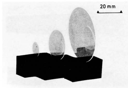
Fig. 6. YAG:Ce<sup>3+</sup> single-crystal transparent screens.
