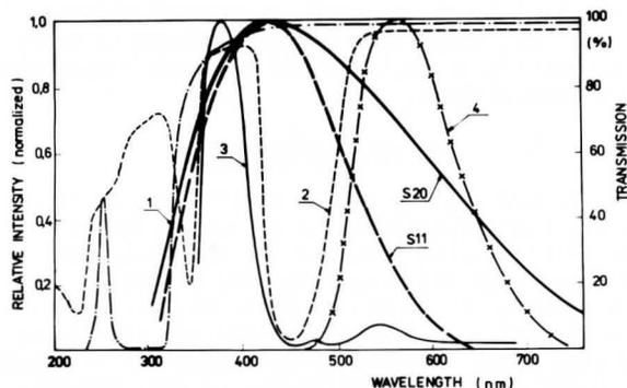
Fig. 1. Absorption and emission spectra of single-crystal scintillators with cathode radiant sensitivity of used photomultipliers (S 11, S 20). 1 - transmission of  $YAP:Ce^{3+}$ , 2 - transmission of  $YAG:Ce^{3+}$ , 3 - emission of  $YAP:Ce^{3+}$ , 4 - emission of  $YAG:Ce^{3+}$ .
