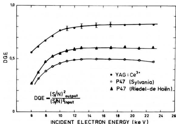
Fig. 3. The detector DQE plotted as a function of the incident primary electron energy. Powder screen density of P 47  $2 \text{ mg cm}^{-2}$ .
