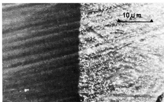
Fig.10. Backscattered electron image. The same position as Fig. 9. Left-hand side - copper (atomic number 29), right-hand side - Cu-Zn alloy (mean atomic number 29.2), specimen current  $1 \times 10^{-10}$  A, accelerating voltage 25 kV, tilt  $0^\circ$ .
