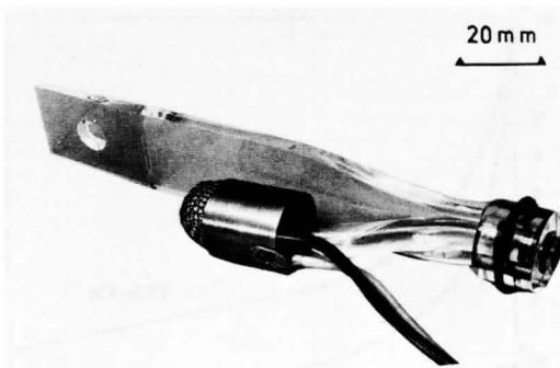
Fig.8. SE and BSE detector with YAG:Ce<sup>3+</sup> single crystal (without metal coating).
