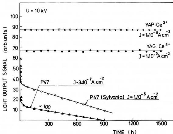
Fig. 5. Light output signal versus excitation time of electron primary beam with 10 keV energy.  $J$  - current density of electron primary beam incident on the scintillator,  $U$  - accelerating voltage.
