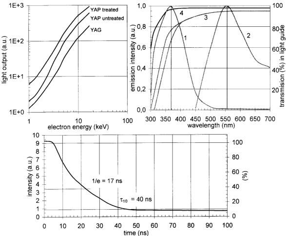
YAG single crystal scintillator is widely and excellently used for the detection of backscattered electrons in SEM. (3). Nevertheless, the YAP single crystal, that was developed according to the last technology, can replace YAG and create BSE detector with improved detection properties.
